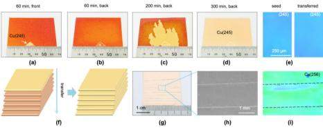
Fig.3-1-39 Replication preparation of single-crystal copper foil with targeted facet
