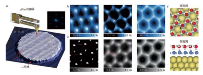
Fig.3-1-9 Schematic diagram of experimental setup, AFM experimental results and simulation of twodimensional ice, and atomic model of two-dimensional ice "interlocking" structure.
