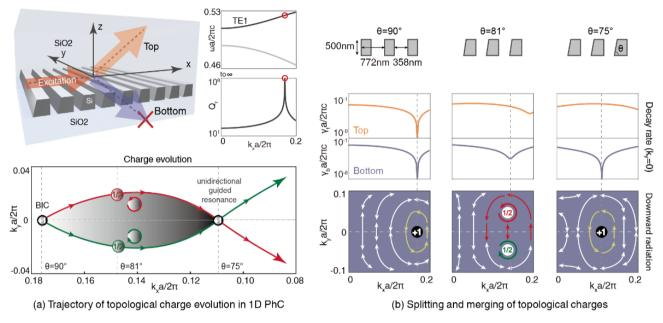
Fig. 3-1-48 Unidirectional guided resonance from manipulating the evolution of topological charges
