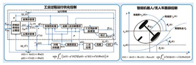
Fig. 3-1-49 Application of linear quadratic optimal control
