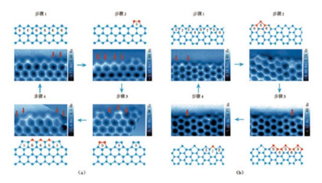
Fig.3-1-10 The "bridging" growth mechanism of the jagged boundary and the "seeding" growth mechanism of the chair-like boundary of the two-dimensional ice.
