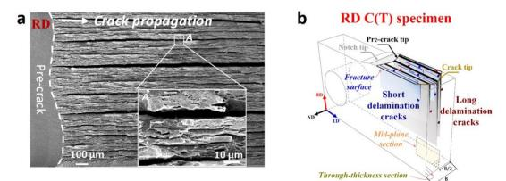
Fig. 3-1-37 The fracture surface and schematic diagram of toughening mechanism of D&P steel. (a) The fracture surface of D&P steel, showing intensive delamination cracks. (b) The schematic diagram of the D&P C(T) specimen, showing the direction of delamination.
