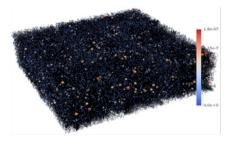
Shale multi-scale pore network model Resolution: 12nm, Throat amount:624537, Pore amount:307820 Physical size: 14.4µm × 14.4µm × 14.4µm
