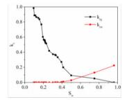
Calculated shale gas-water relative permeability curve based on pore network model
