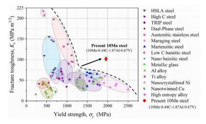
Fig. 3-1-36 Yield strength-toughness and of the present breakthrough D&P steel compared with other existing high strength metallic materials.
