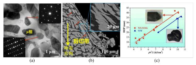
Fig.3-1-4 A new type of tungsten high-entropy alloy with outstanding self-sharping capability: (a) ultra strong µ phase precipitations, (b) shear-banding induced by high strain gradient, (c) this new alloy achieves the 10-20% larger penetration depth than 93W.
