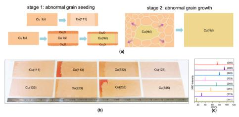
Fig.3-1-38 Preparation of large-size single-crystal copper foil library
