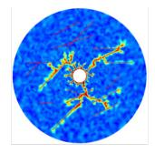
Extension of dissolved wormholes caused by acid fracturing in shale gas reservoir
